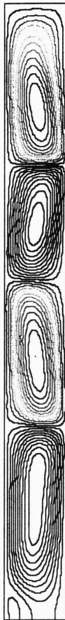
Figure 4. Stream function for water in 2-mm gap at Ta = 600 .
